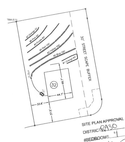
•Keep Tanks and Drain lines 10' from property lines.
