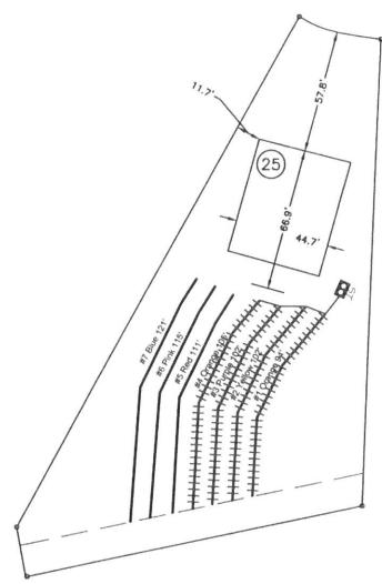
\*Keep Tanks and Drain lines 10' from property lines.
