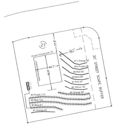
\*Keep Tanks and Drain lines 10' from property lines. \*Not a Survey \*Not a guarantee of a septic permit.
