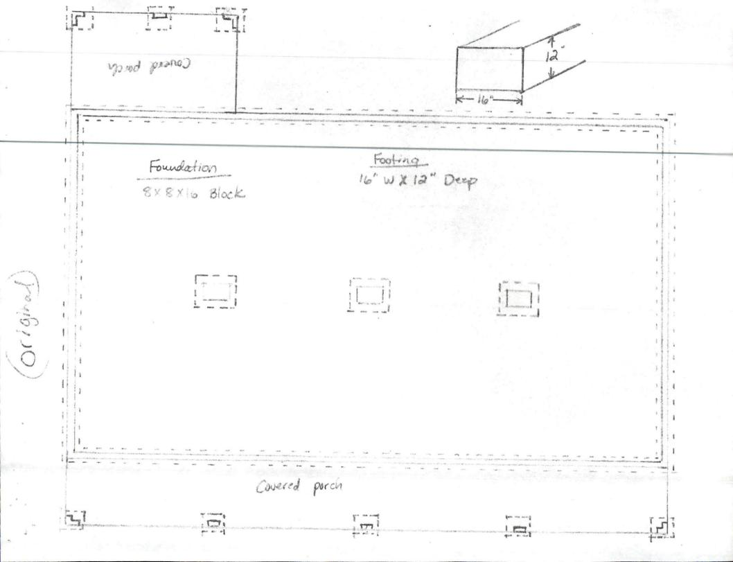
3) 2X10 Sirders W/ 2x2 Ledger 24" craw space 2x6 seal 16"x16" Block Peir on ay"x2y"x12" footer 2 x10 Floor joist 2 16" O.C. 2x/2 Header
