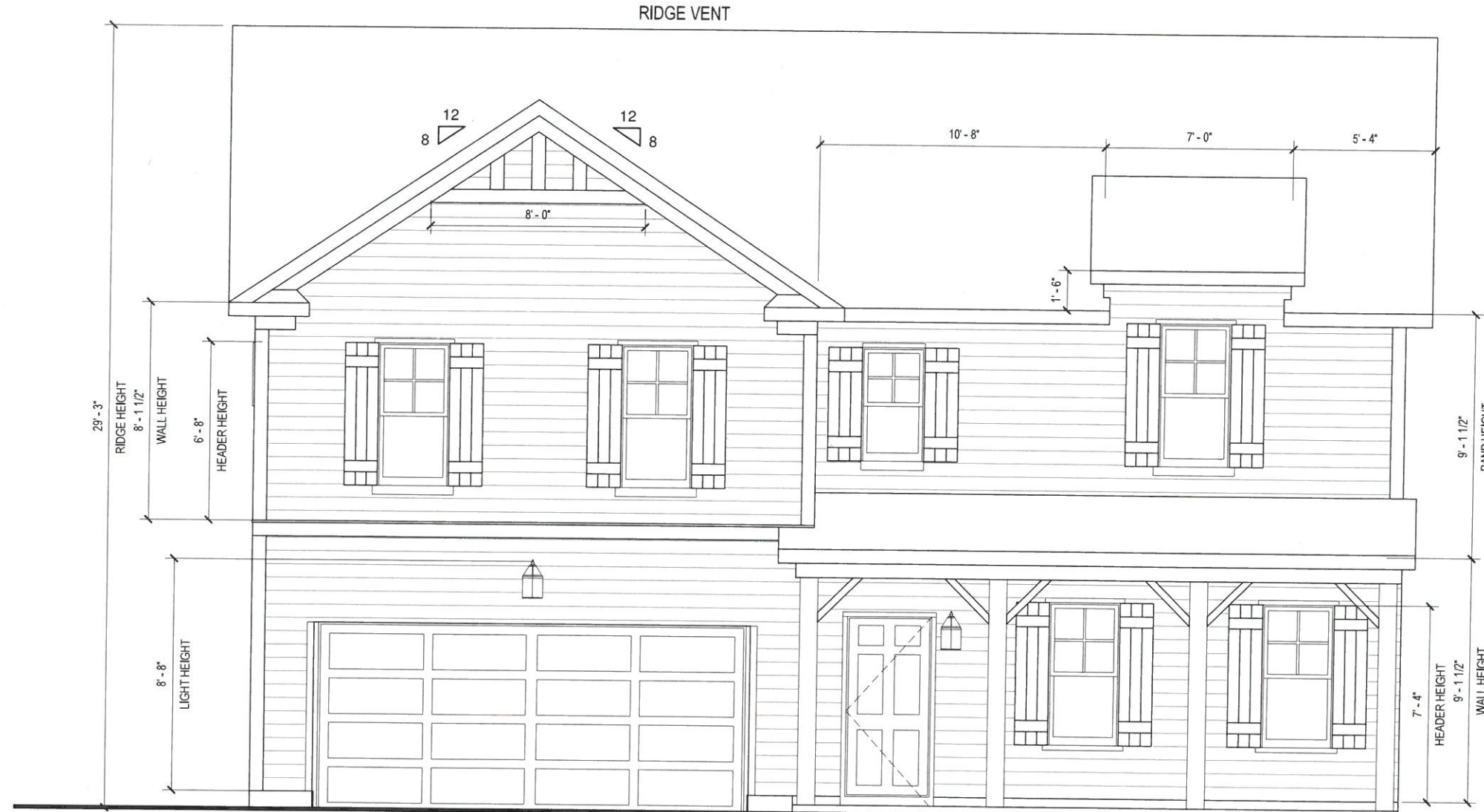
A FRONT ELEVATION - THE GRIFFIN 4346 - C 3/16" = 1'-0"
