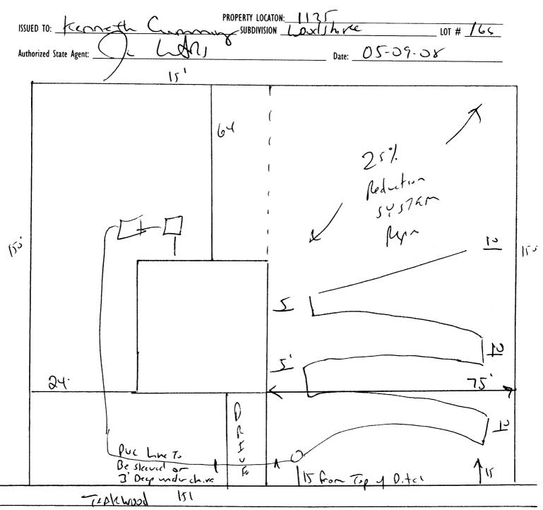
Meet Doute for Final Layort Maintain All Jet OAiler (NC 2ppl) Line To be Sleeved or 3' Deep under Deve WAX Zostall 245 1 25% Reduction System At 18"
