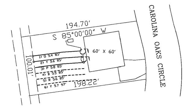
LINE LENGTHS SHOWN ON THIS PAGE MAY BE LONGER THAT THE SPECIFIED DESIGN LENGTHS. TO ENSURE PROPER INSTALLATION PAY ATTENTION TO SPECIFICATIONS AND TAPS SHEETS CONNECTED WITH DESIGN. SEPTIC, PUMP TANKS AND ALL DRAINLINES NEED TO BE 10' OFF PROPERTY LINES.
