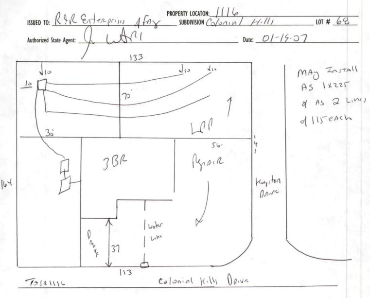
Meet onsite STUB OUT Plembing where shown Maintain All Set Backs Enstall 3×75 of 25% Reduction System At 18"
