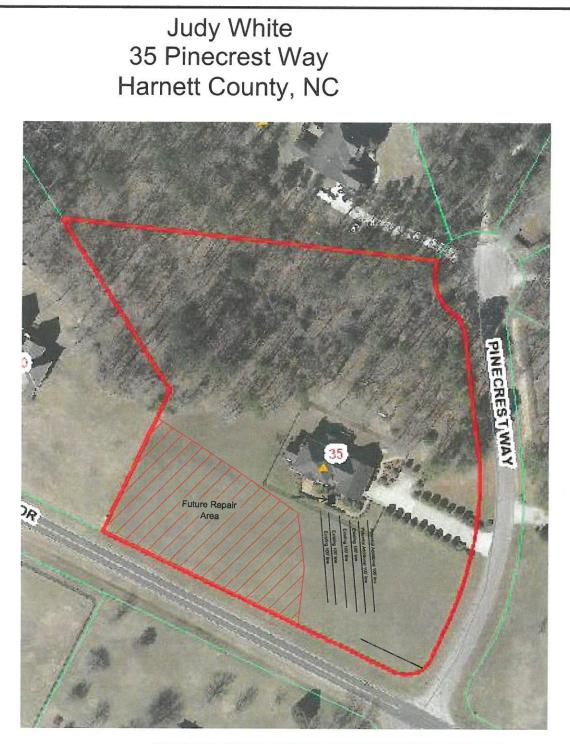
\*System could be upgrade to accomodate a 5-Bedroom home by installing a 1200 gallon tank and adding two-100' septic trenches
