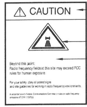
5 CAUTION-RF SIGN (YELLOW) 12" WIDE X 18" HIGH
