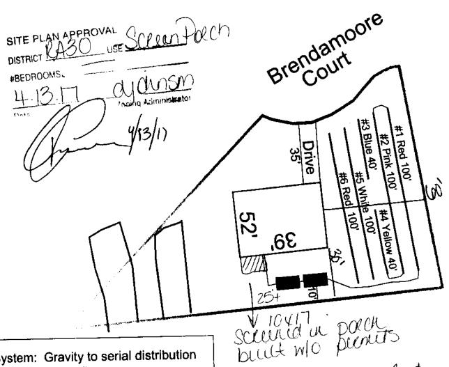
System: Gravity to serial distribution
