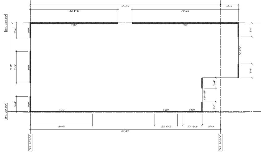
SECOND FLOOR BRACED WALLS
