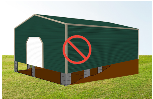
No Installs on Unlevel Land
