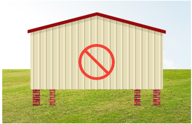
No Installs on Stacked Blocks
