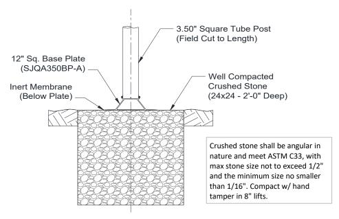
**Base Plate Over Crushed Stone**
