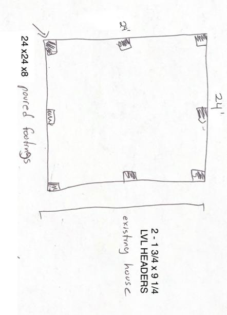
6x6 post will be anchored to concrete
