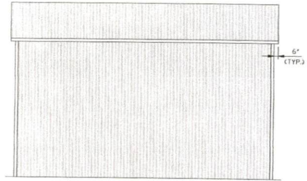
TYPICAL SIDE ELEVATION VERTICAL ROOF/SIDING
