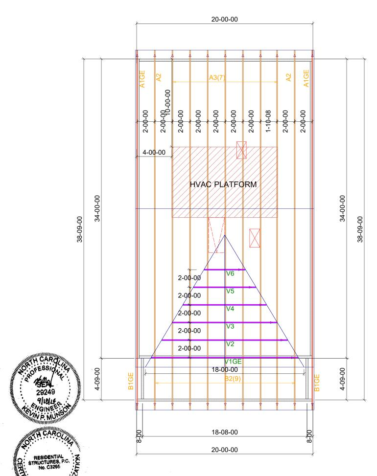
TRUCTURES, P.C. C. No. C3286 RESIDENTIAL STRUCTURES, RC. 3410 N. Devideon St. Charlotte, N.C. 28205 Seal For Structure Cally ROOF TRUSS LAYOUT
