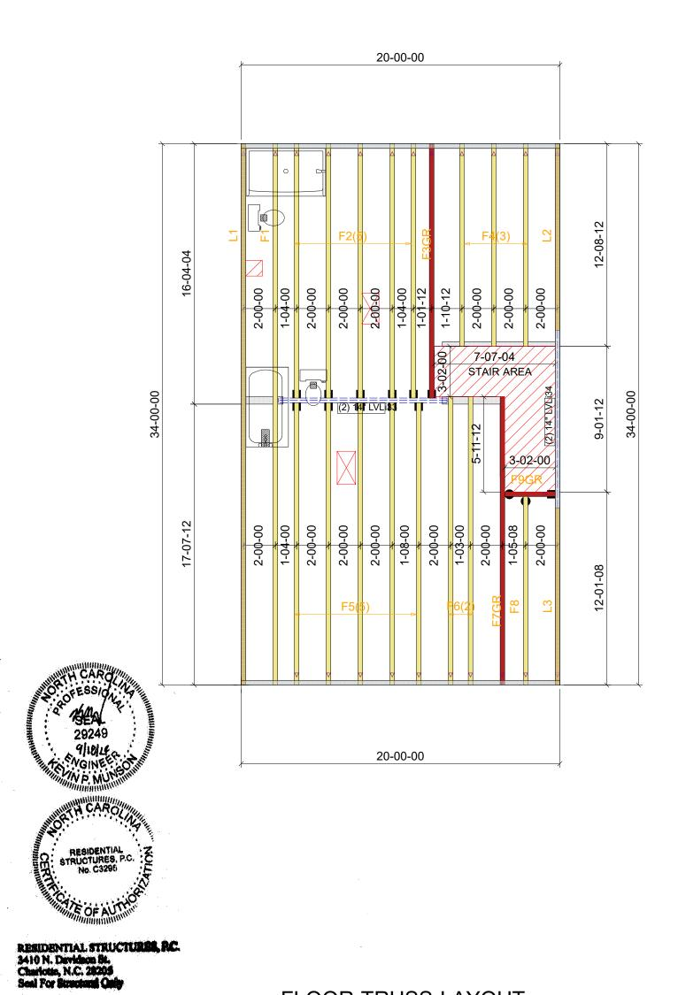
FLOOR TRUSS LAYOUT SCALE: 3/16" = 1'-0"
