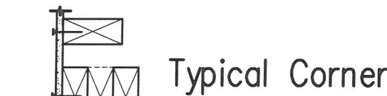
B Corner Framing Detail
