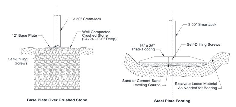
Crushed stone shall be angular in nature and meet ASTM C33, with max stone size not to exceed 1/2" and the minimum size no smaller than 1/16".
