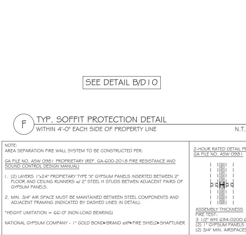
F TYP. SOFFIT PROTECTION DETAIL WITHIN 4'-0" EACH SIDE OF PROPERTY LINE N.T.S.
