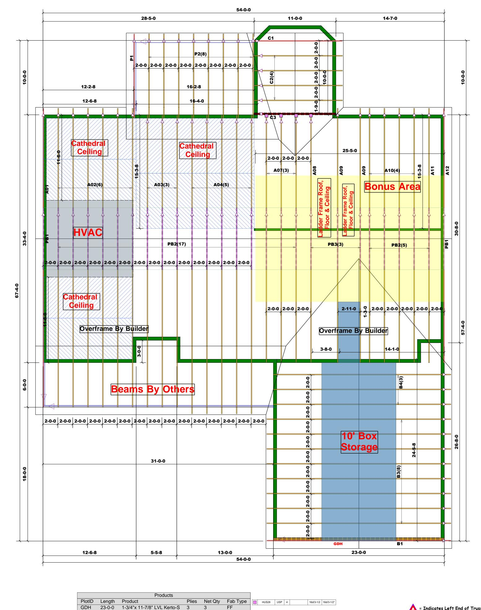
**Truss Placement Plan** SCALE: 1/\*4"=1'
