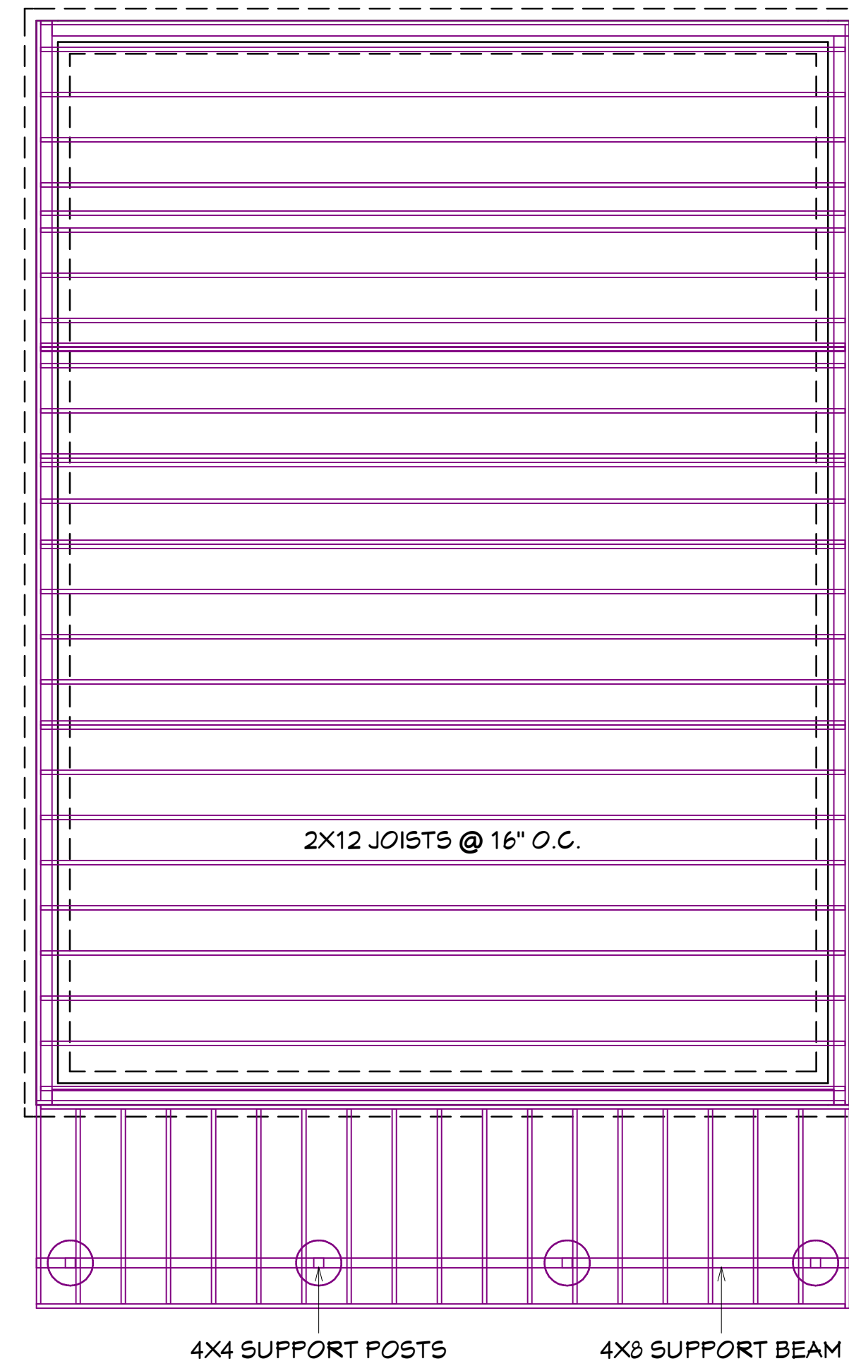
FLOOR FRAMING PLAN SCALE: 1/4" = 1'
