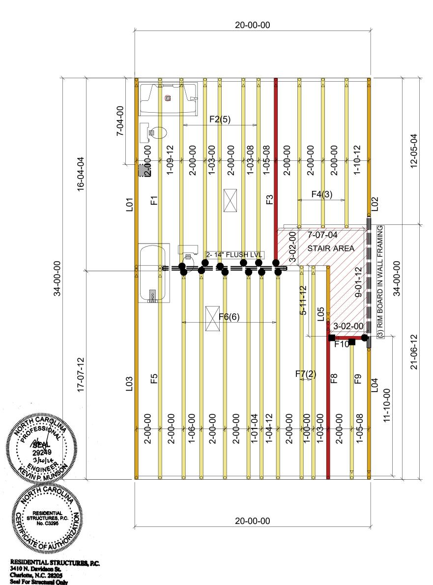
Floor Truss Layout SCALE: 1/4"=1'
