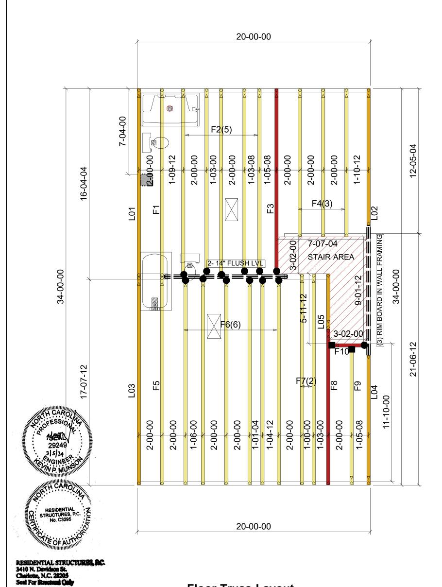
Floor Truss Layout SCALE: 1/4"=1'
