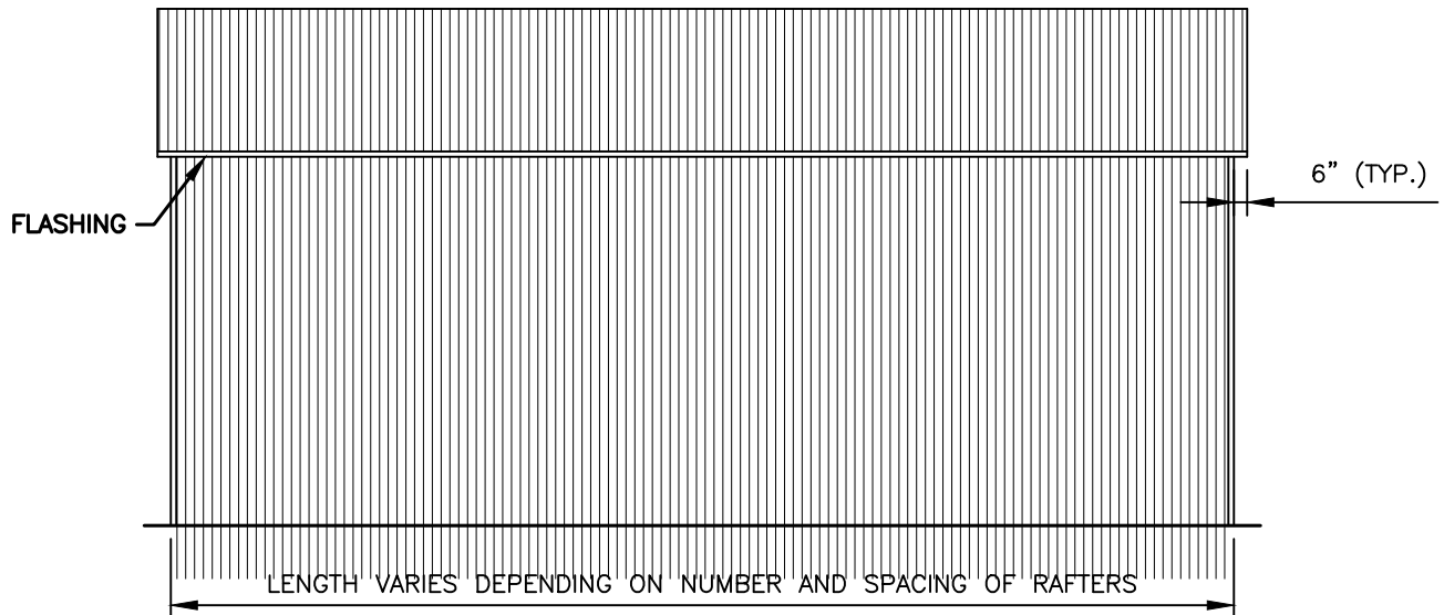
TYPICAL SIDE ELEVATION - VERTICAL ROOF / SIDING
