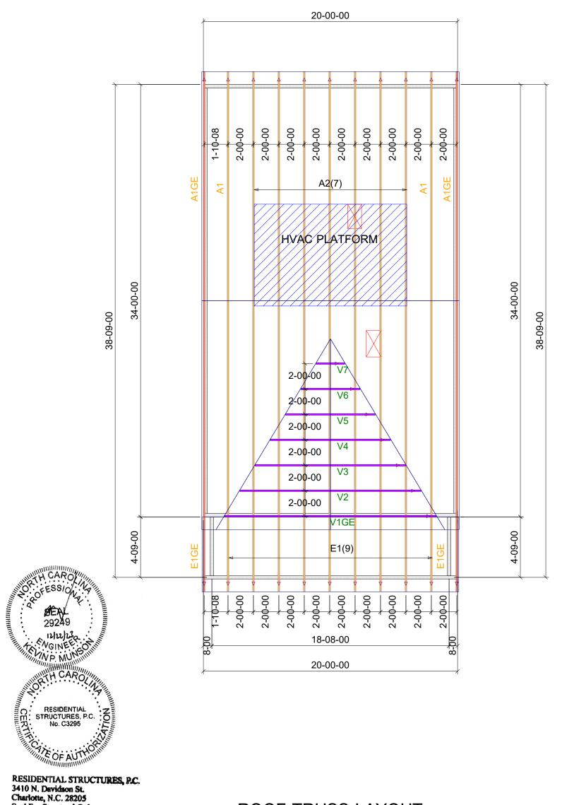
ROOF TRUSS LAYOUT SCALE: 3/16" = 1'-0"
