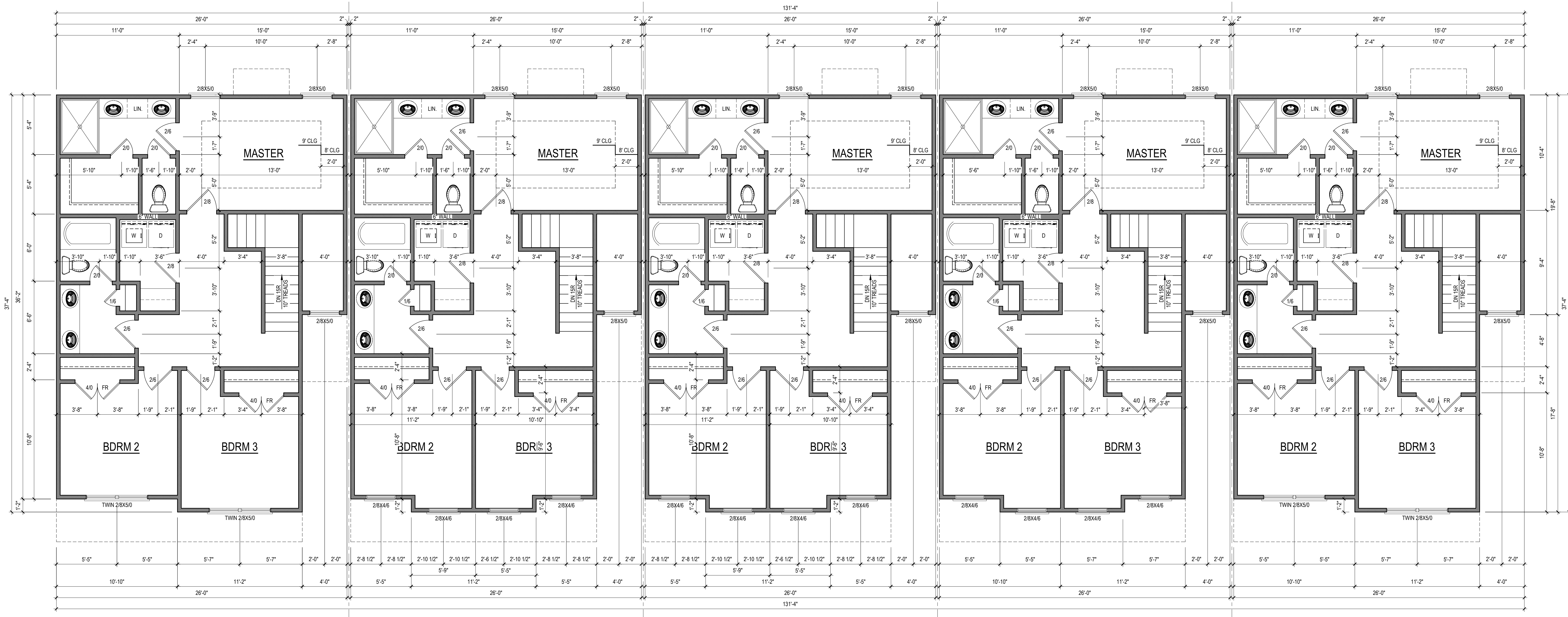
SECOND FLOOR PLAN - ELEV. A 1/4" = 1'-0" CLG. HGT. = 8'-0"
