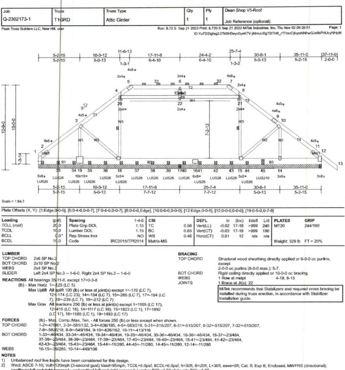
cantilever left and right exposed; end vertical left and right exposed; Lumber DOL=1.60 plate grip DOL=1.60
