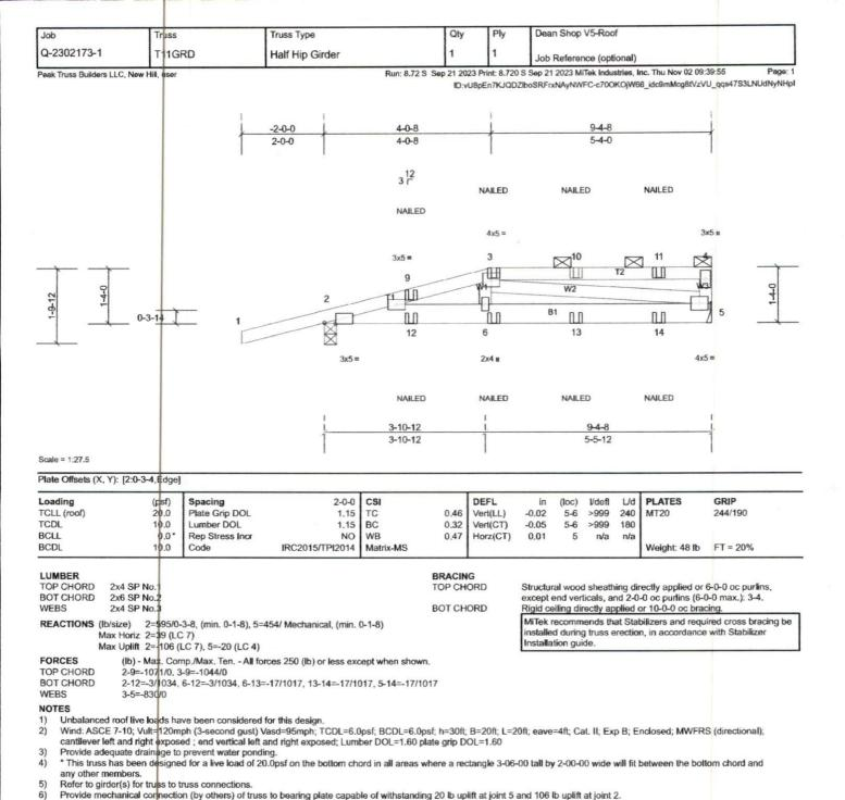
This truss is designed in accordance with the 2015 International Residential Code sections R502.11.1 and R802.10.2 and referenced standard ANSI/TPI 1.
