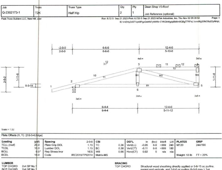
**BOT CHORD** 2x4 SP No. 2x4 SP No.3 Structural wood sheathing directly applied or 5-6-15 oc purlins, except end verticals, and 2-0-0 oc purlins (6-0-0 max.): 3-4. Rigid ceiling directly applied or 10-0-0 oc bracing.
