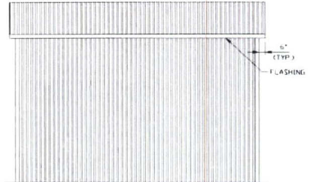
TYPICAL SIDE ELEVATION VERTICAL ROOF/SIDING
