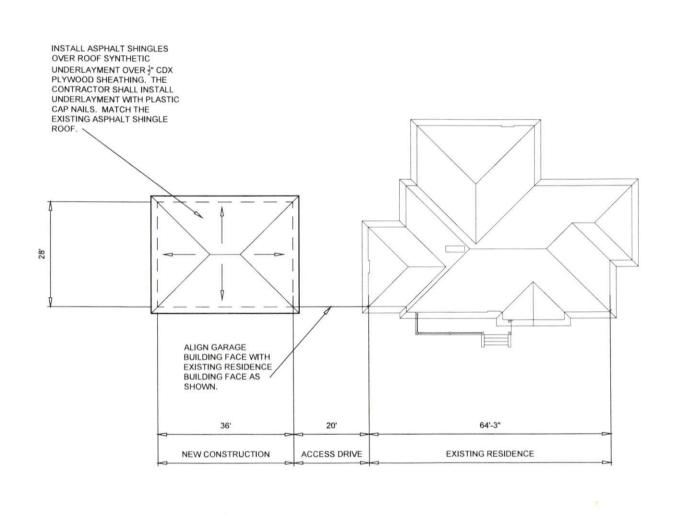
SITE PLAN SCALE: 1' = 300' DESIGN DEVELOPMENT-NOT FOR CONSTRUCTION
