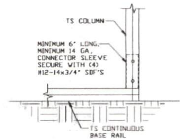
8 COLUMN/BASE RAIL CONNECTION DETAIL SCALE: NTS
