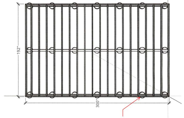
round footings shall be 128sq inches minimum equivalent (13 in diameter min)
