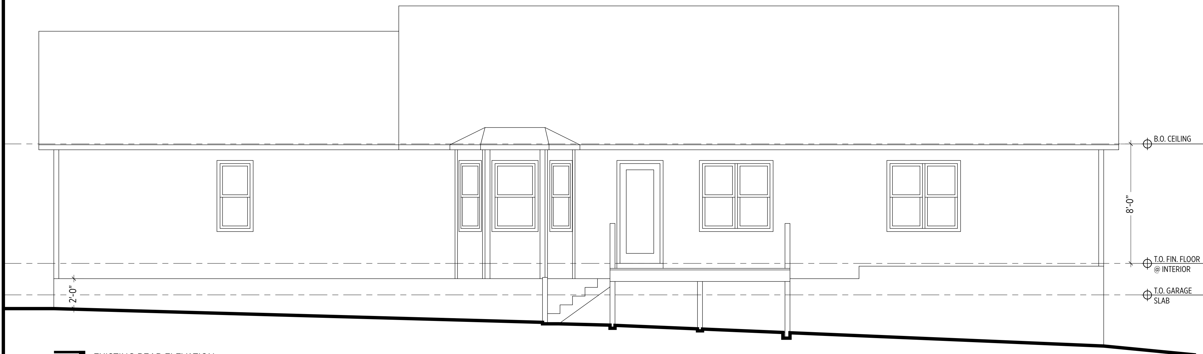
1 EXISTING REAR ELEVATION SCALE: 1/4" = 1'-0"
