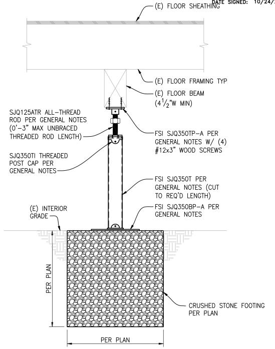
REF PLAN FOR LAYOUT & INSTALLATION REQ'S INSTALL PER MFR RECOMMENDATIONS
