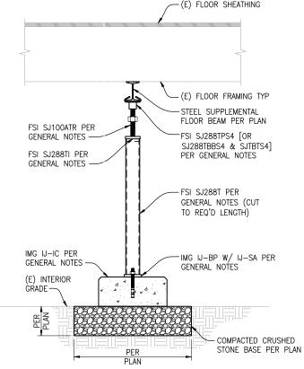
Note: Section above is a general representation of smartjack system, refer to plan for layout and project specific details.
