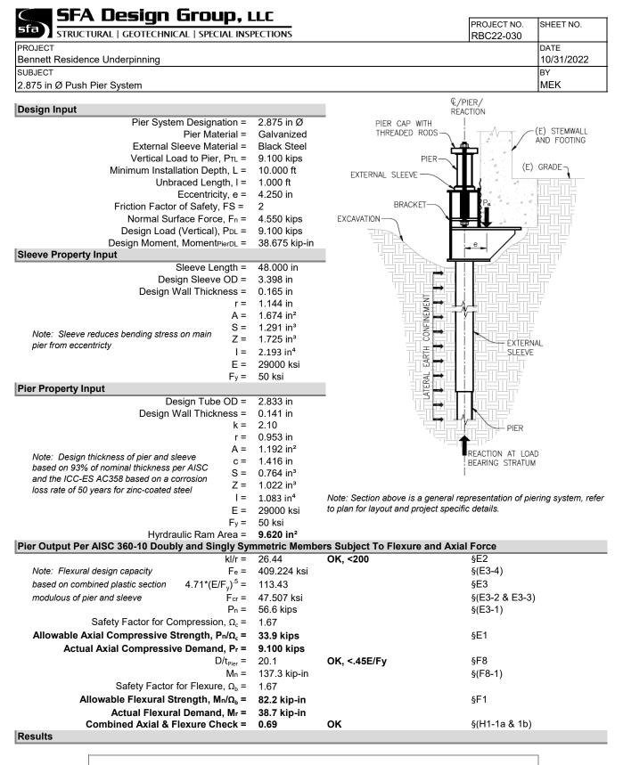
Max Load To Pier = Design Load = 9100 lb 2.875" Diameter Pipe Pier with 0.165" Thick Wall 3.5"Diameterx48" Long Pipe Sleeve With 0.216"ThickWall Minimum 10'-0" Installation Depth And Minimum 2000 psi Installation Pressure Minimum ¼" Foundation Lift During Installation
