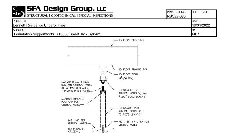
Note: Section above is a general representation of smartjack system, refer to plan for layout and project specific details.
