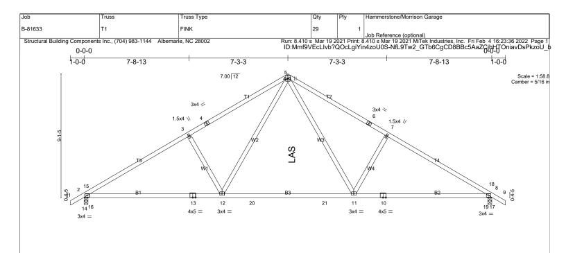
0-0-0 0-0-0 10-1-14 10-1-14 9-8-5 1-0-0 30-0-0 1-0-0 LOADING (psf) TCLL 20.0 SPACING-1-4-0 1.15 CSI. DEFL in (loc) -0.37 11-12 PLATES GRIP 244/190 Plate Grip DOL 20.0 0.60 Vert(LL) >980 360 MT20 TCDL 10.0 Lumber DOL 1.15 BC 0.71 Vert(CT) -0.65 11-12 >552 240 WB BCLL 0.0 Rep Stress Incr NO 0.36 Horz(CT) 0.05 8 n/a n/a Code IRC2015/TPI2014 BCDL 10.0 Weight: 144 lb FT = 20%
