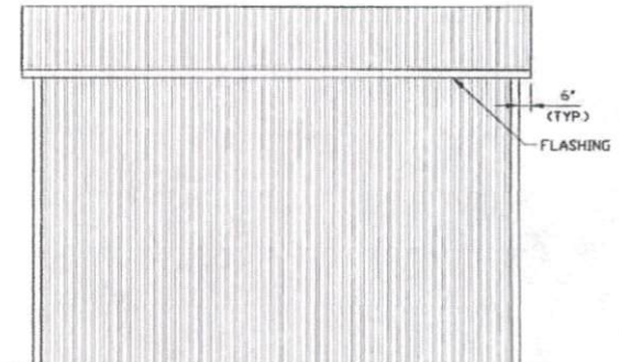
TYPICAL SIDE ELEVATION VERTICAL ROOF/SIDING SCALE: NTS
