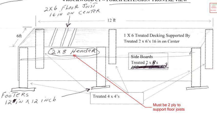
Because of the Ground Slope, The Left Side of the Deck Will Be 15 inches Above the Ground Level.
