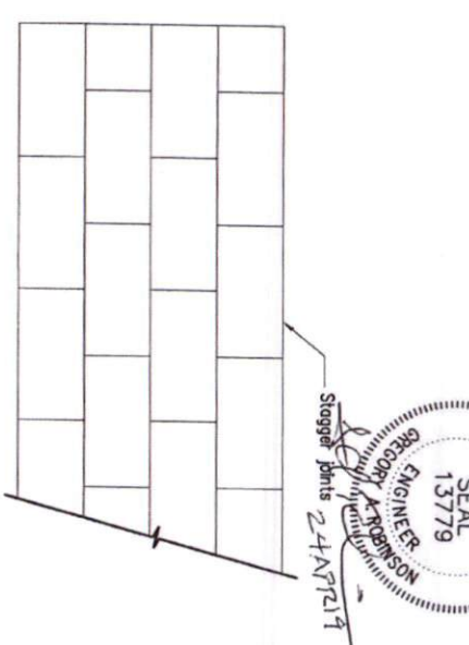
D Sheathing Joint Pattern
