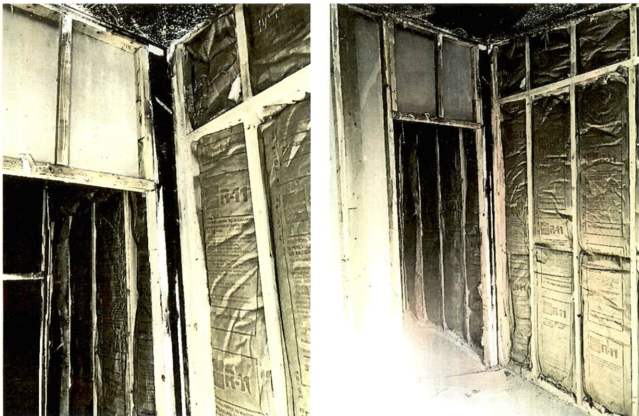
Figure 2. Representation of some of the burned members
