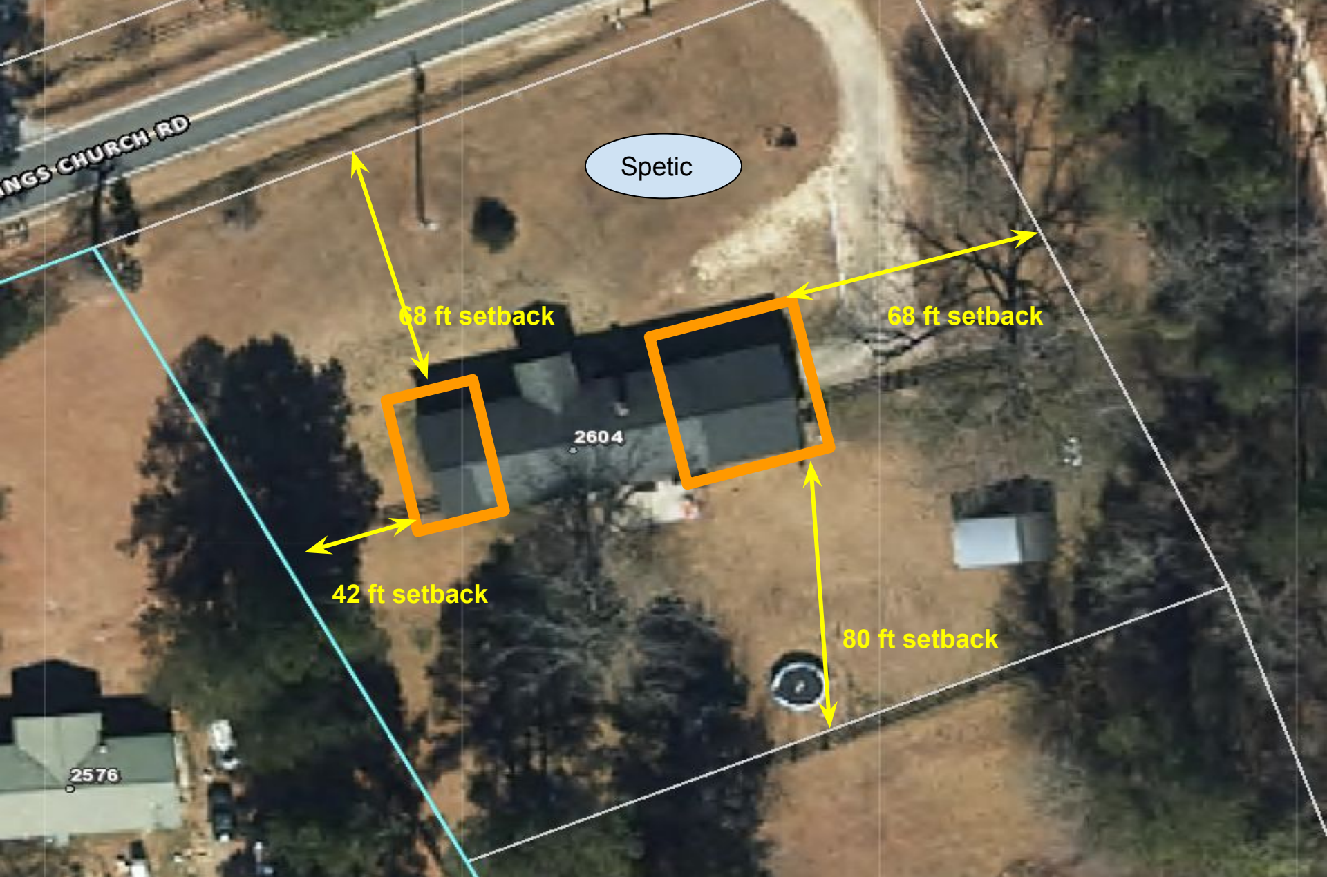
New Additions are shown in Orange boxes. Change in roof color indicates new area. Left side Closet enlargement by 8 ft. Right side Utility room and carport, 24 ft
