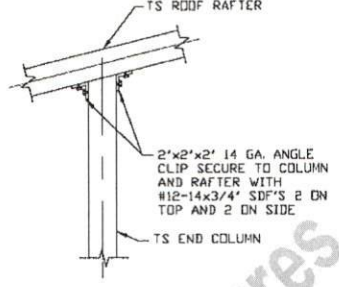
4 END COLUMN/RAFTER CONNECTION DETAIL SCALE: NTS
