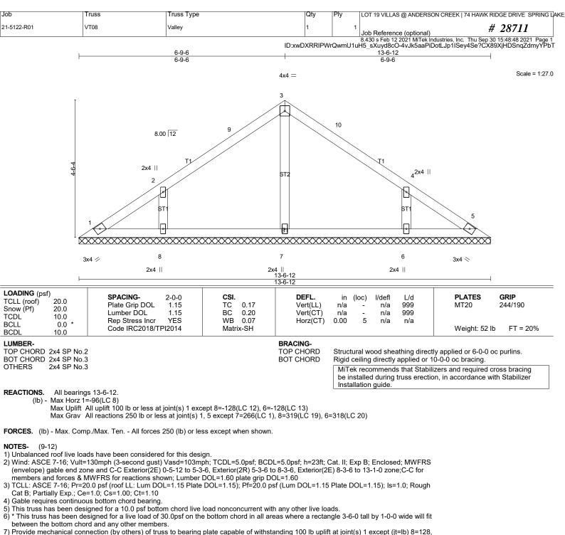
7) Provide mechanical connection (by others) of truss to bearing plate capable of withstanding 100 lb uplift at joint(s) 1 except (jt=lb) 8=128, 6=128.
