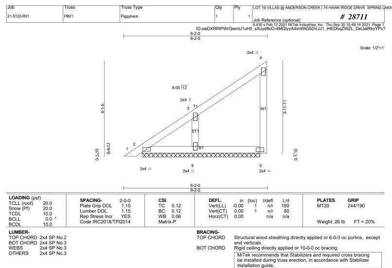
REACTIONS. (lb/size) 5=94/5-1-0 (min. 0-1-8), 2=97/5-1-0 (min. 0-1-8), 6=259/5-1-0 (min. 0-1-8) Max Horz 2=136(LC 12) Max Uplift5=-37(LC 12), 6=-106(LC 12) Max Grav 5=99(LC 20), 2=97(LC 1), 6=273(LC 20)
