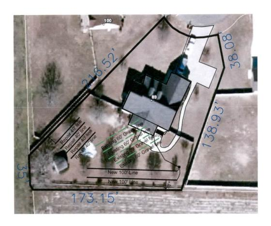
\*Do Not Cut, Fill, or Alter Drainfield or Repair Area \*Comply with all setbacks
