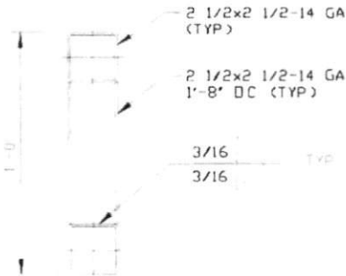
HEADER DETAIL FOR OPENINGS 12'-0" < LENGTH ≤ 20'-0" SCALE: NTS
