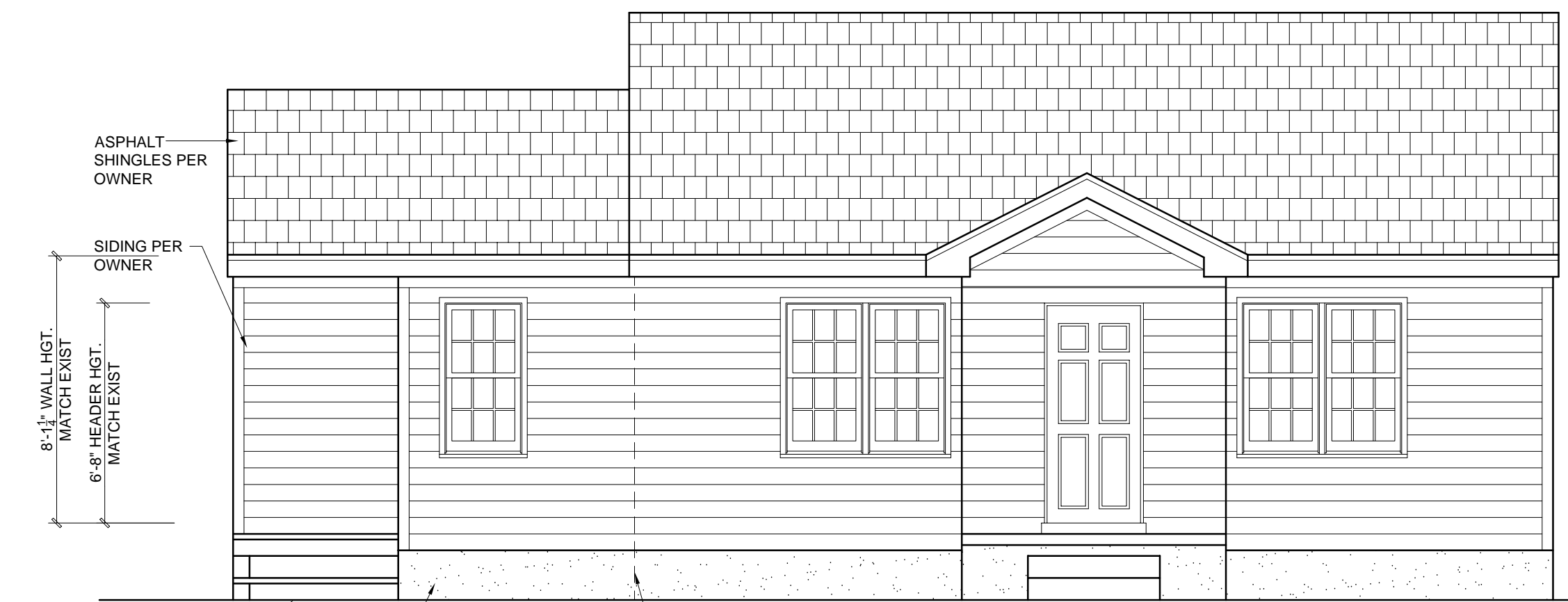
FRONT ELEVATION 22X34 PRINTS SCALE: 1/4"=1'-0" 11X17 PRINTS SCALE: 1/8"=1'-0"
