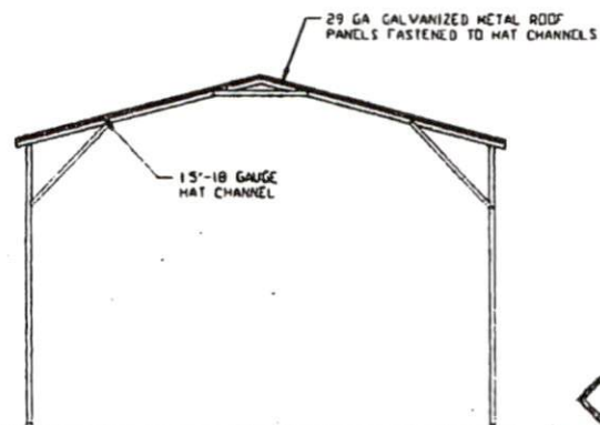
TYPICAL SECTION VERTICAL ROOF/SIDING OPTION SCALE: NTS
