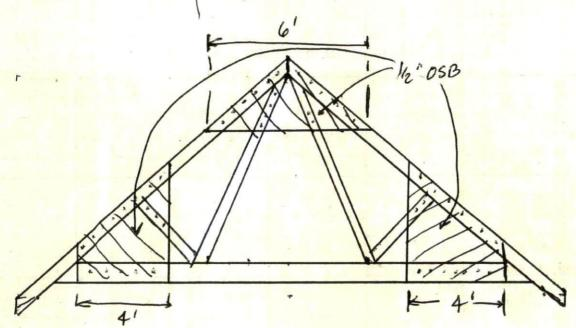
FRASTEN &" OSB TO EACH SIDE OF THE EXISTING TRUSSES WITH CONSTRUCTION ADHESIVE AND 1-1/2" WAILS OR SCREWS SPACED AT 8" CONSTRUCTS
