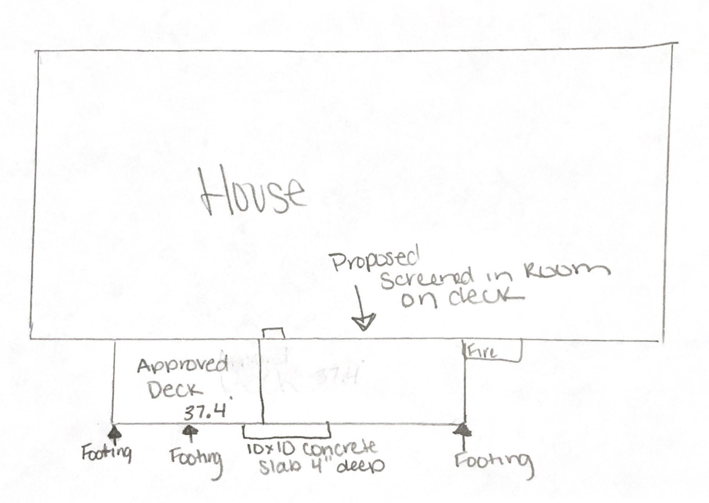
12" # All Footings are sono tube and are deep 2Pt un top of concrete Slah deck is triple beamer Support
